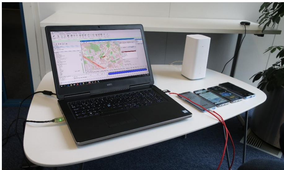
Figure 12: Stationary measurement setup with Nemo Outdoor and a set of 4G/5G terminals.
