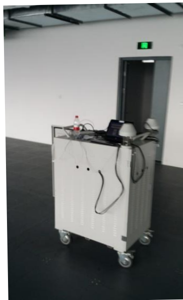
Figure 134: Mobile and stationary measurement points with two terminals connected to a laptop running the measurement tools.
