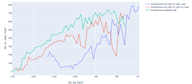
Figure 3. PDCP comparison among three cases: isolated base station, interference without scrambling and interference with scrambling.
