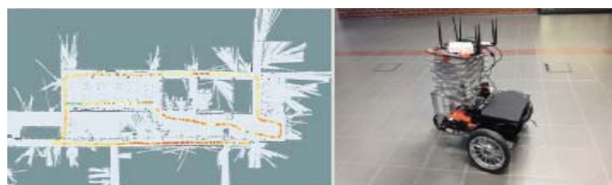
Fig. 6. (a) Floor map including measured strength values; (b) mobile robot used for the IPS platform
