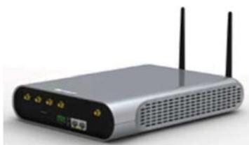
Fig 5. RSU components used in the V2X trials in China twinning project. The message exchange benefits between RSU and in-vehicle OBUs are the trial goals.
