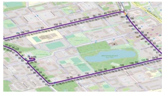
Fig 12. Latencies measured in the local MEC service in the L1 test field
