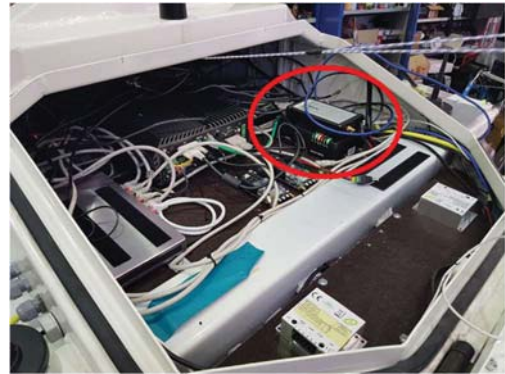
Fig 2. On-Board Unit (OBU) in eLvira test vehicle.
