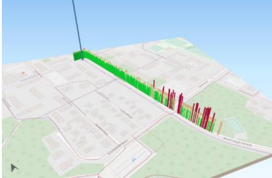
Figure 52: Latency contour plot (LTE-V2X): msg interval 20 ms, tx RSU at blue location (green < 26ms, red > 36ms). The driving speed in this case is 15-25 km/h
