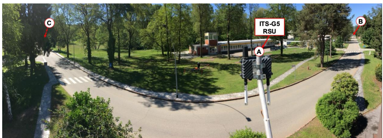
Figure 70: Line-of-sight road section (points B-A-C, length ~ 650 m) in the Ispra trial (ITS-G5 field test)
