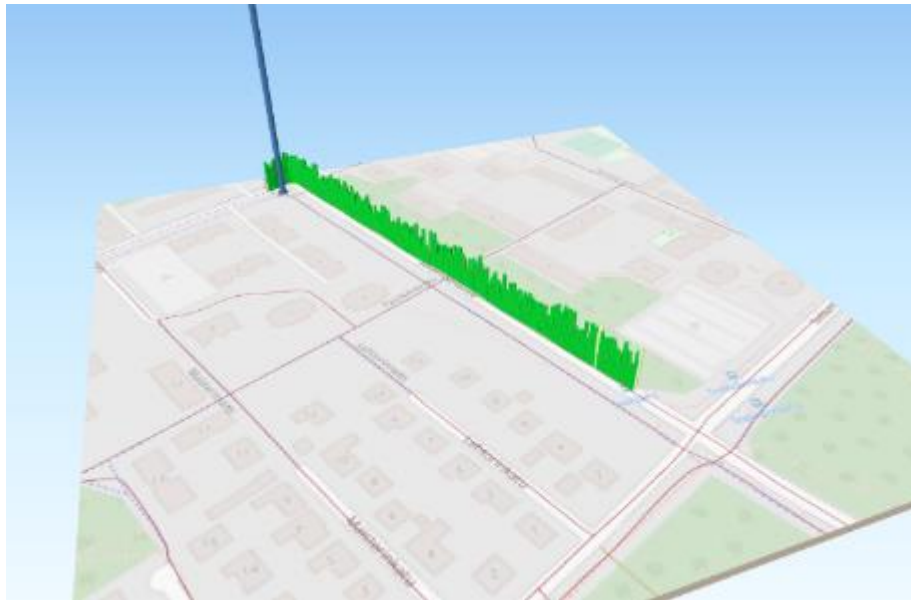
Figure 60: Latency: Automated driving V2X, msg size 250B, tx RSU in blue location (green < 26ms, red > 36ms).
