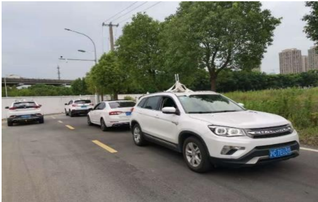
Figure 45: The OBU is placed on the top of the test car. The height of the antenna is about 1.5 m
