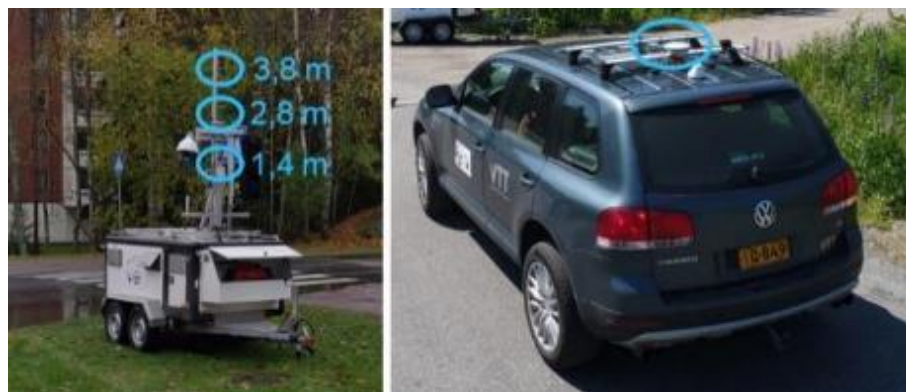
Figure 50: Antenna installations in the LTE-V2X trials. Left: antenna installations on the trailer; Right: the 5G and LTE-V2X antennas of the test vehicle "Marti" located on the roof.
