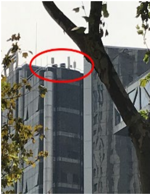
Fig.4 the 2.6 GHz and 4.9 GHz base station on the roof of the opposite building and the location of the selected measurement points
