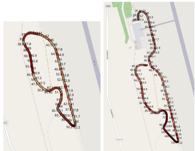
Fig. 5. Ping measurements at the 5G test site. Left: without collaborative sensor data; Right: LiDAR data delivered over the 5G network.
