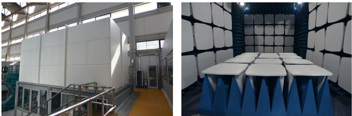
Figure 9: The small shielded anechoic chamber at the Joint Research Centre Ispra
