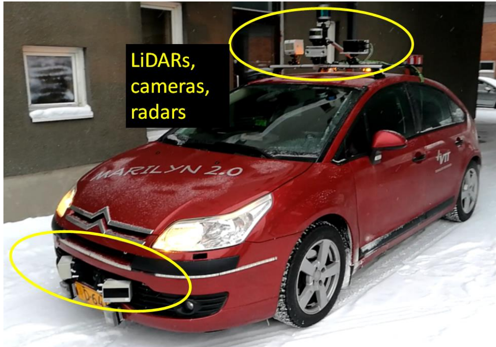
Figure 3: Instrumented and automated Marilyn demo vehicle with on-board sensors
