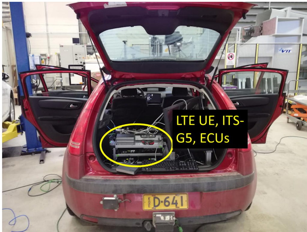
Figure 5: The Embedded Control Units (ECU) and communication units (Sierra Wireless LTE and ITS G5) are in the trunk of the car
