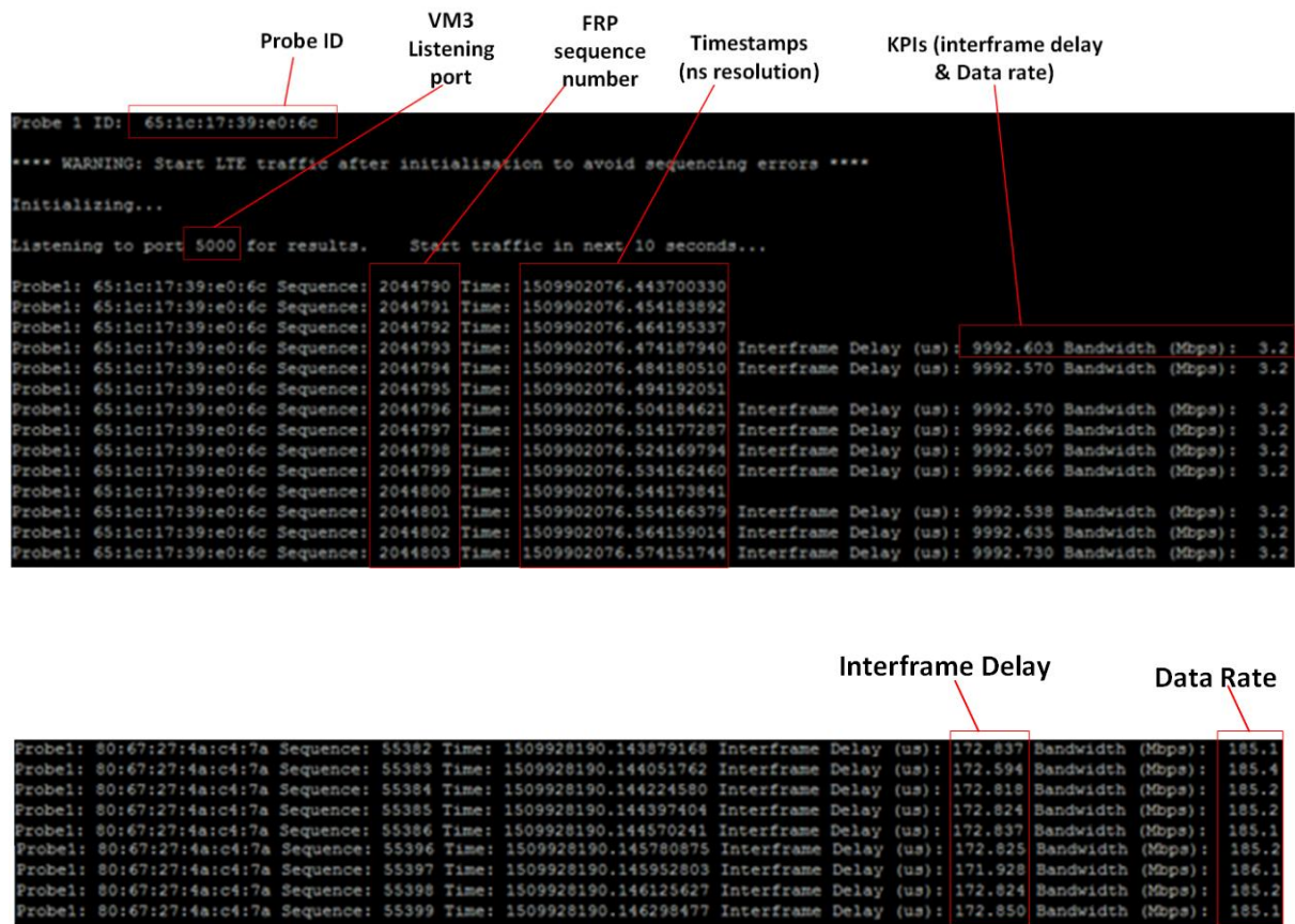
Figure 20: Screen capture of live performance monitoring with generated inter-frame delay and data rate KPIs. (Bottom) Monitoring with a source generating traffic with a throughput of 0.2 Gbps (approx). Annotations show the probing metadata and the generated KPIs.
